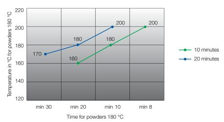
Light colour shades can cause a shift. The maximum temperature is around 210 °C. All data refer to object temperature.
